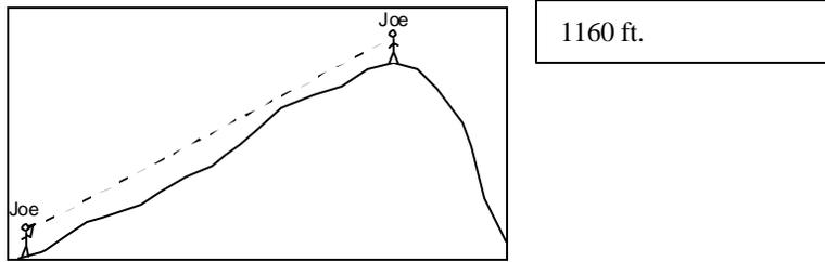
7. (9.1) Set up and complete the differential level notes for the information shown in the accompanying illustration. All back sights are shown to the left of the instrument diagrams and fore sights are shown to the right. All units are feet. Be sure to show your arithmetic check. (5 pts)
